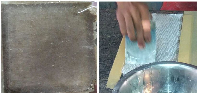
Fig. 5: Fabrication of Glass-Rice Husk-Vinyl Ester hybrid composite
