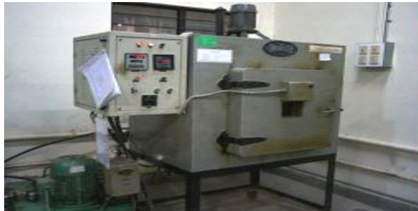
Fig 6: Post curing oven
